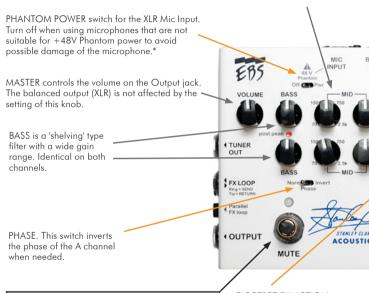
MUTE FOOT SWITCH. Mutes the balanced outputs and the master output.
