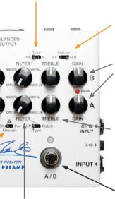
FILTER works in conjunction with the TYPE switch for each channel. Choose between High Pass (HP) or Notch, and set the value with the Filter knob. Default position is the FILTER knob turned down to Off and the Type switch set to HP. Set the values individually for the A and B channel
